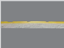
Top - .75mm thick Polyvinyl Bottom - 1/4" thick Visco Elastic
